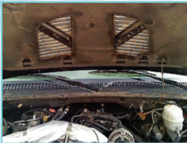
Under-the-hood view of hood louver in a Tahoe.
