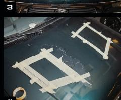
3 & 4. After you have the louvers where you want them, put a piece of masking tape around all four sides of each of the louvers to mark the locations. Then remove the louvers and put another strip of 1" masking tape around the inside edge of the tape that marked the edge of the louvers. This will mark out the lines you need to cut on.
