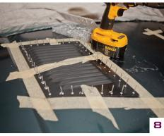
8. Place a pop rivet down into each hole to confirm that all the holes line up and are the correct size.
