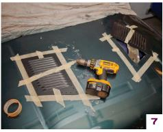
7. Remove the inner row tape and put the hood louvers back into place. Securely tape the louvers onto your hood so you can start drilling the hole for the pop rivets. Using the provided drill bit, start drilling out the holes. Use some nails or screws to put into the holes to help hold the louver in place as you drill the rest of the holes.
