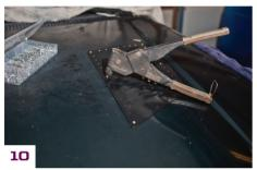
10. After the paint dries, rivet the hood louvers down. Start with the corner holes, then move to the center holes to allow the louver to match the hood curves. You're done!
