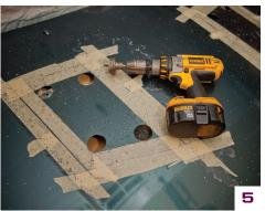
5. This is the most important step. Cover your windshield with a thick cloth. If this is not done you will end up with lots of little metal shavings melted into your glass. To start the surgery on the hood it is wise to use a hole saw on the four corners of each section you are going to cut out. This will give you a nice rounded corner that will be more rigid than a square corner.
