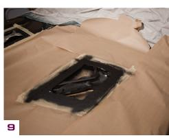
9. Mask off the rest of your hood because it is time to paint the exposed metal around the sides of the holes you just made.
